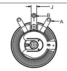
Variable Resistors Top View (FVR) Dimensions
