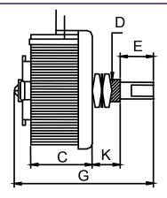
Variable Resistors Side View (FVR) Dimensions
