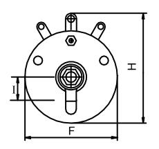
Variable Resistors Bottom View (FVR) Dimensions
